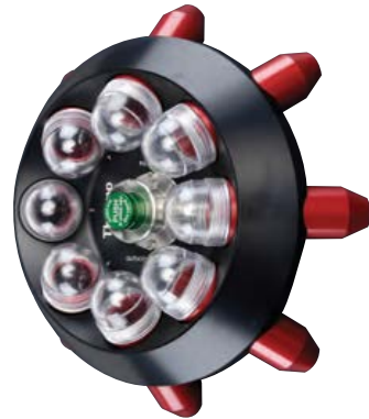
8 x 50 Individually Sealed Fixed Angle Rotor, 45° , R max 143 mm
