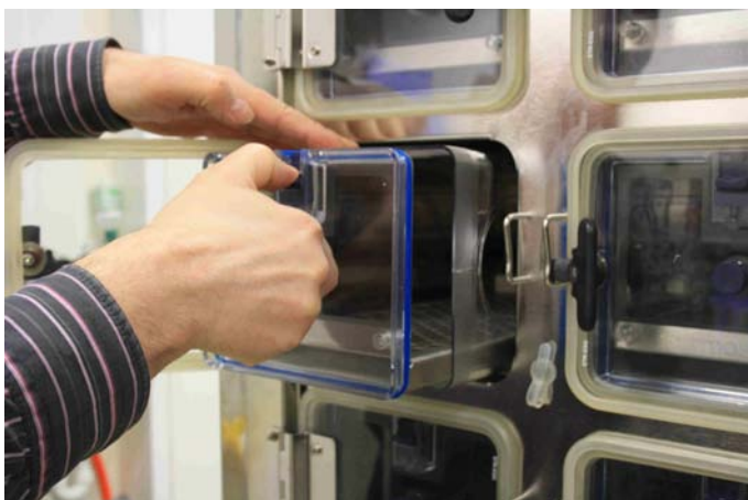
samples access inside the chamber with transport cover
