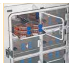
Gas Tight Inner Doors with Split Shelves
