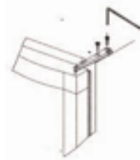
4. Remove the top hinge while holding the door
