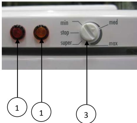
The freezer is controlled with the thermostat knob.
