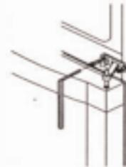
7. Remove the kick panel. Unscrew nuts and pivot, remount on the opposite side of the angle iron.
