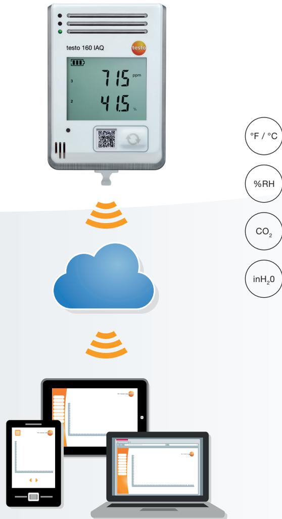
The testo 160 IAQ Wi-Fi Data Logger is ideal for rapid deployment in monitoring indoor air quality. Using internal sensors for temperature, humidity, CO<sub>2</sub>, and atmospheric pressure, the testo 160 IAQ accurately determines the air quality of your desired area and communicates it within your secure network using the web-based testo Saveris 2 Cloud.
