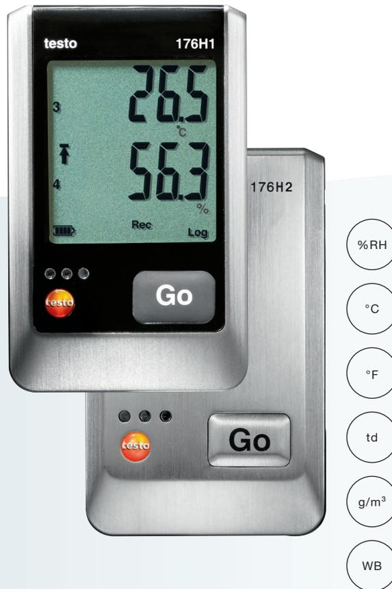
The Testo engineered logger for parallel measurement of two temperature / humidity points with external humidity probes. Some of many applications include humidity chambers, incubators, produce coolers and laboratory applications.
