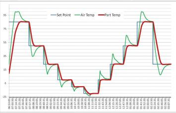
Air temperature is biased higher/lower in a precise manner for the fastest response at the DUT.
