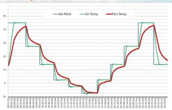
DUT never quite reaches the temperature setting. Longer test time if you actually wait for the DUT to reach Set Point.
