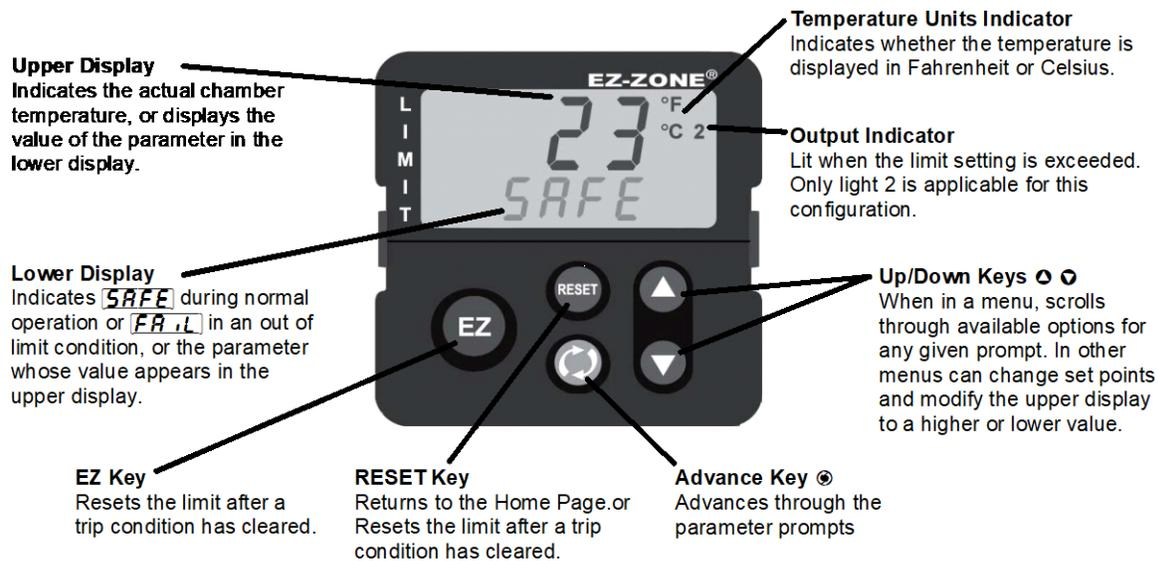
Figure 4.1 – Limit Controller Keys and Displays
