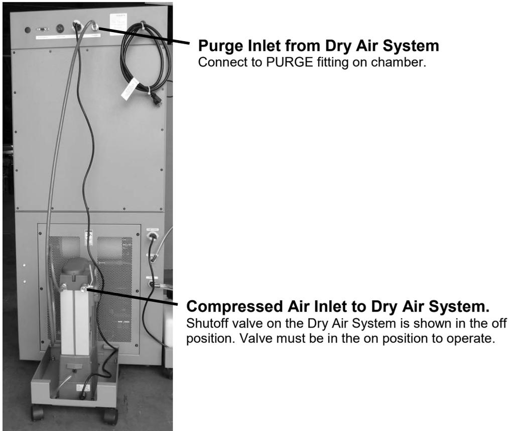
Figure 5-1 – Dry Air Purge System Installation (typical)
