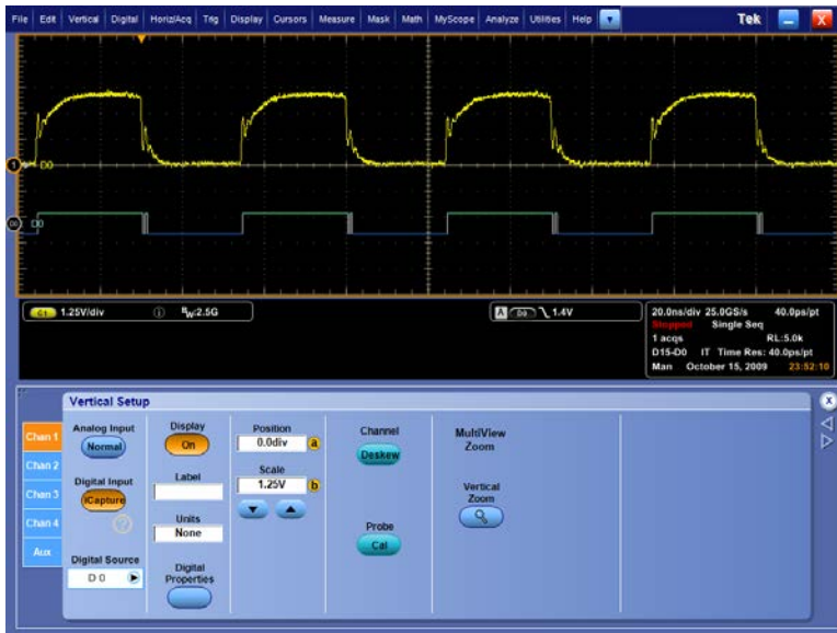
Figure 6. Edge ringing causing digital transitions.
