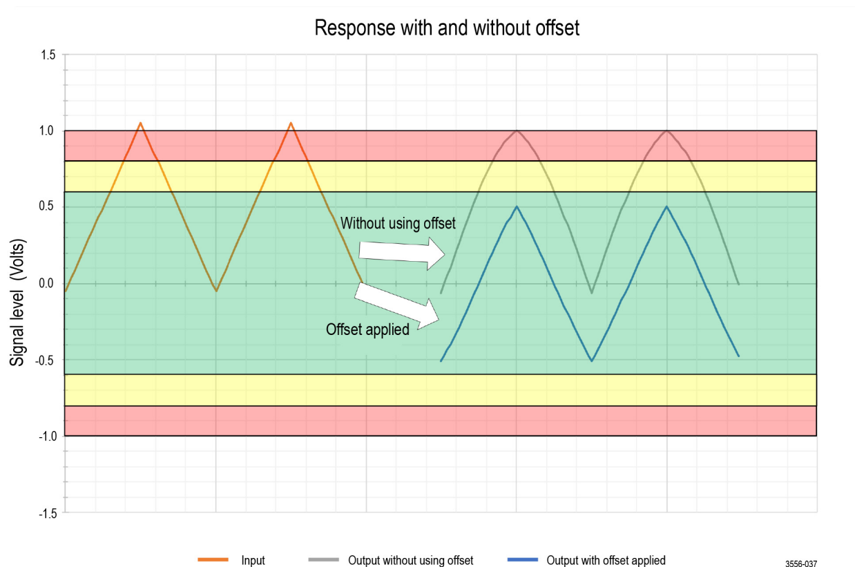
Figure 17: Use of input offset to improve signal fidelity
