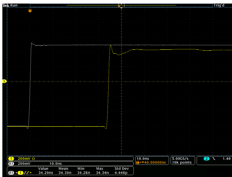
Figure 56: Propagation delay measurement
