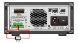
After making the connections, slide the cover over the rear-panel mating connector and wires.
