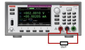
The following illustration shows two-wire (local sensing) DUT connections to the rear panel.
