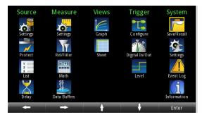
From this screen, you can select source, measure, Views, Trigger, and System setup menus. These menus allow you to choose options to set up your instrument for your applications. Select a menu item by either scrolling using the navigation control or using the arrow keys to highlight an icon. Then press **ENTER**.
