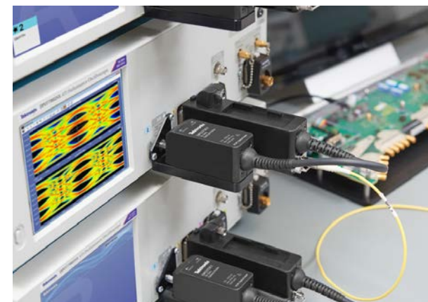
DP070E Series Optical probes using the TekConnect channel on a DP077002SX ATI Performance Oscilloscope.
