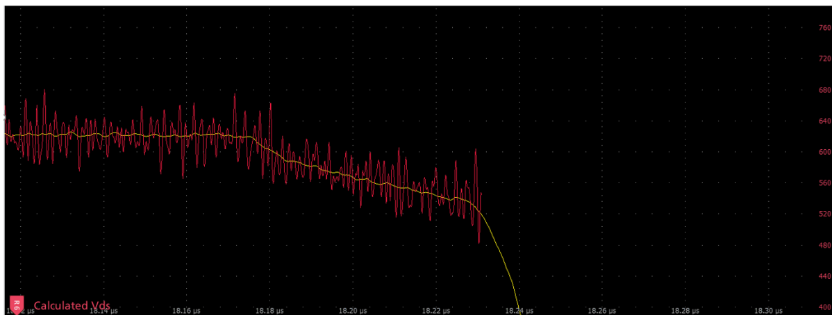
Figure 44: Noisy model of Vds using small differential order filter at turn on transient
