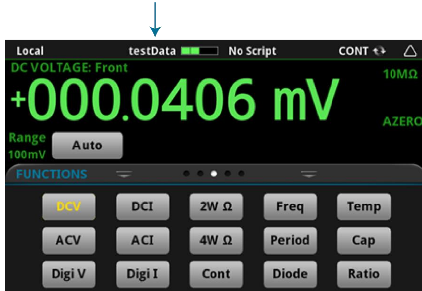
Figure 119: Active buffer indicator
