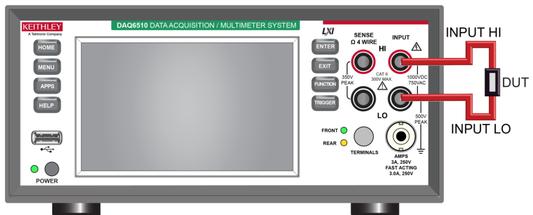
Figure 67: Two-wire DUT connections to the front panel
