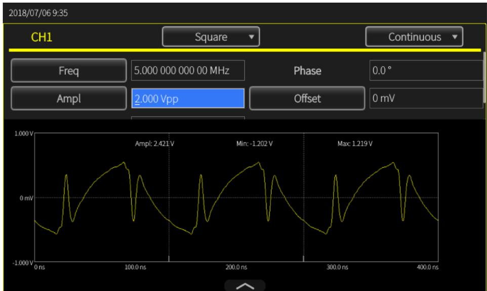
Figure 74: Amplitude 2 VPP - Scope InstaView
