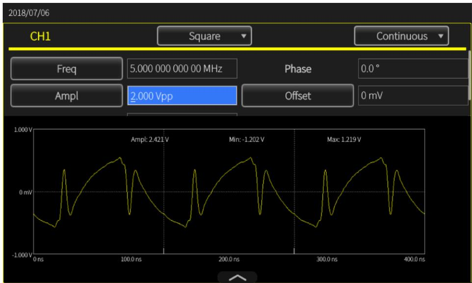
Figure 73: Frequency 5 MHz - scope
