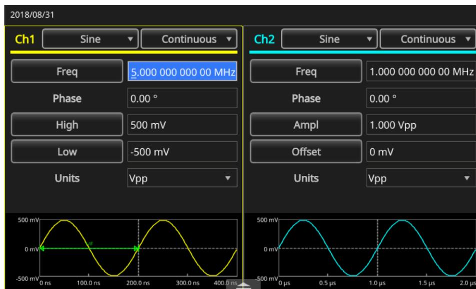
**Figure 45: CH1 frequency 5 MHz**
