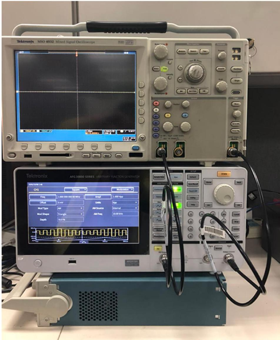
Figure 157: AFG31000 Series connected to an oscilloscope
