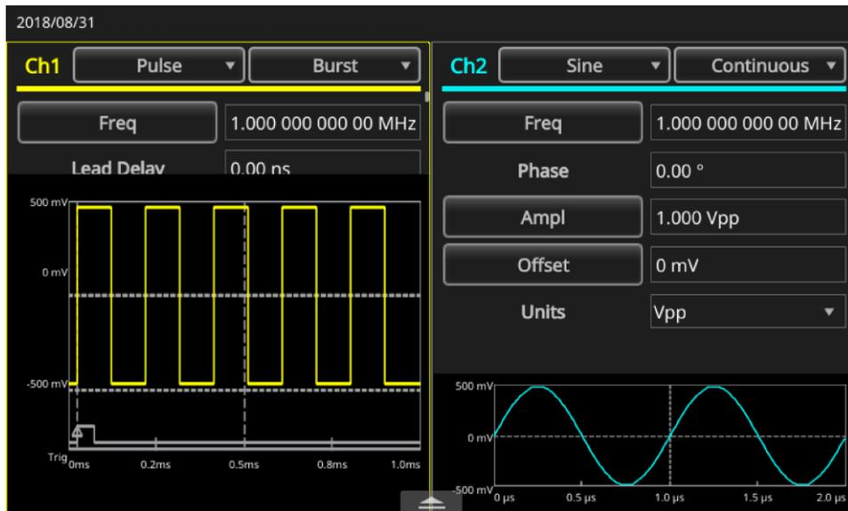
Figure 33: Burst pulse waveform
