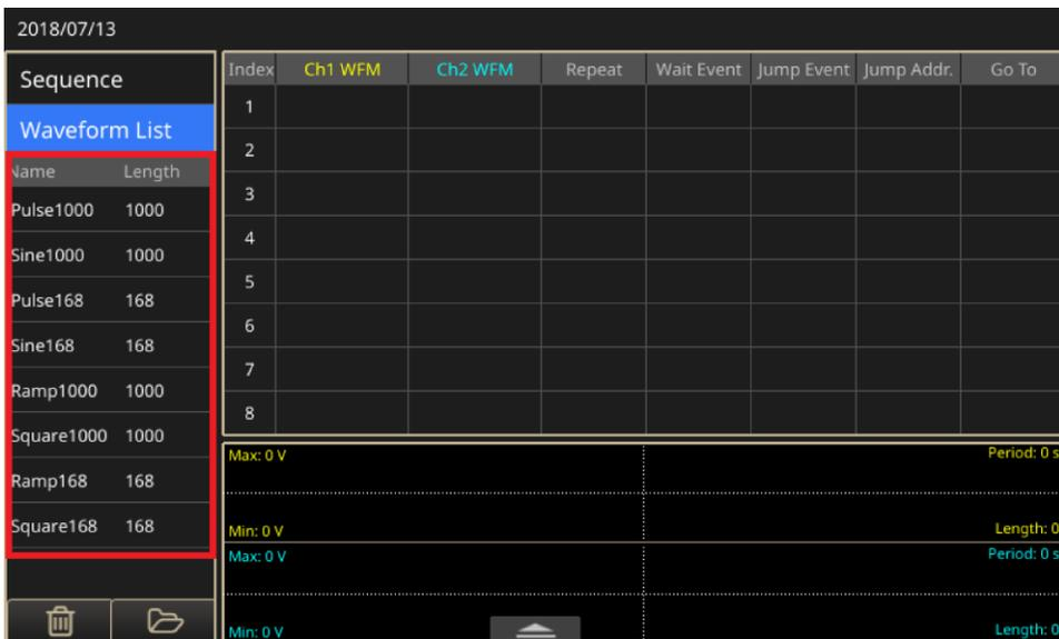
Figure 93: Select from the Waveform List
