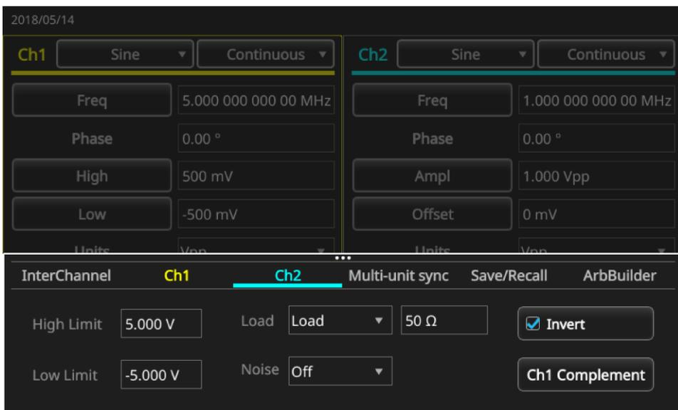
Figure 55: Ch2 tab and CH1 Complement button
