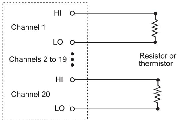
**Figure 9: Four-wire resistance and RTD connections**
