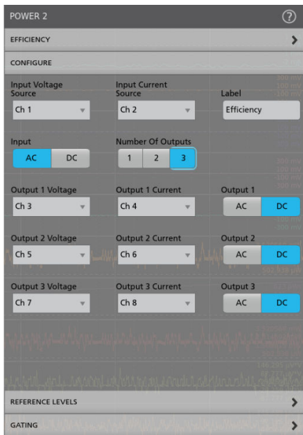
Figure 11: Efficiency measurement configuration lets you test new generation multi-output power conversion devices (AC-DC, AC-AC, DC-DC, and DC-AC)
