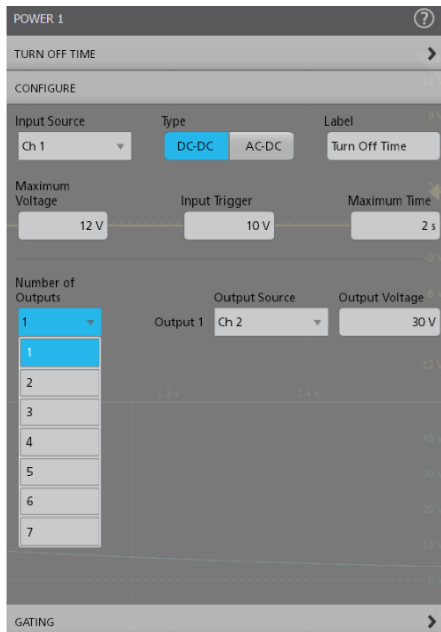
Figure 15: The Turn off time measurement configuration supports multiple outputs
