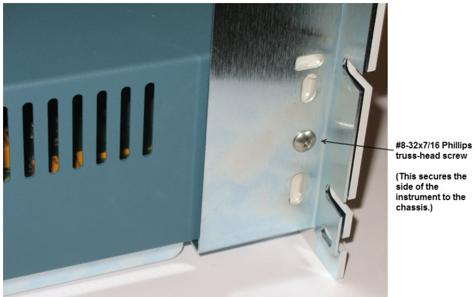
Figure 27: Install the support bracket
