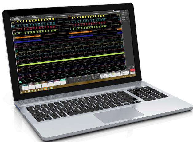
Figure 32: TekScope PC analysis software runs on a Windows computer with the same award-winning user experience as the 4, 5, and 6 Series MSO's
