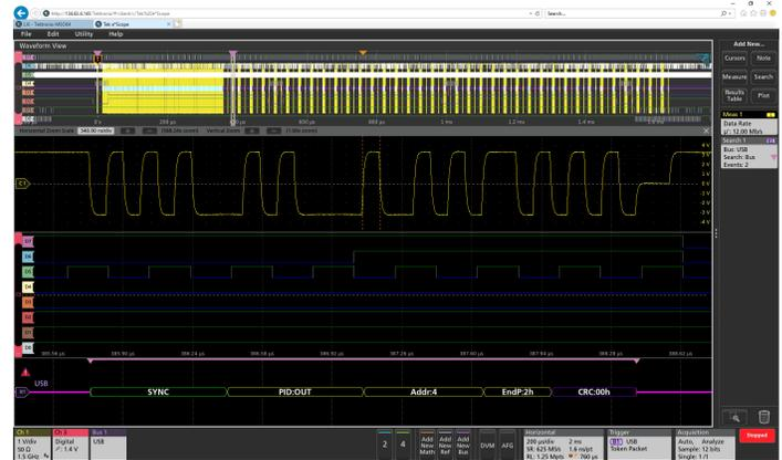
Figure 31: e\*Scope provides simple remote viewing and control using common web browsers.
