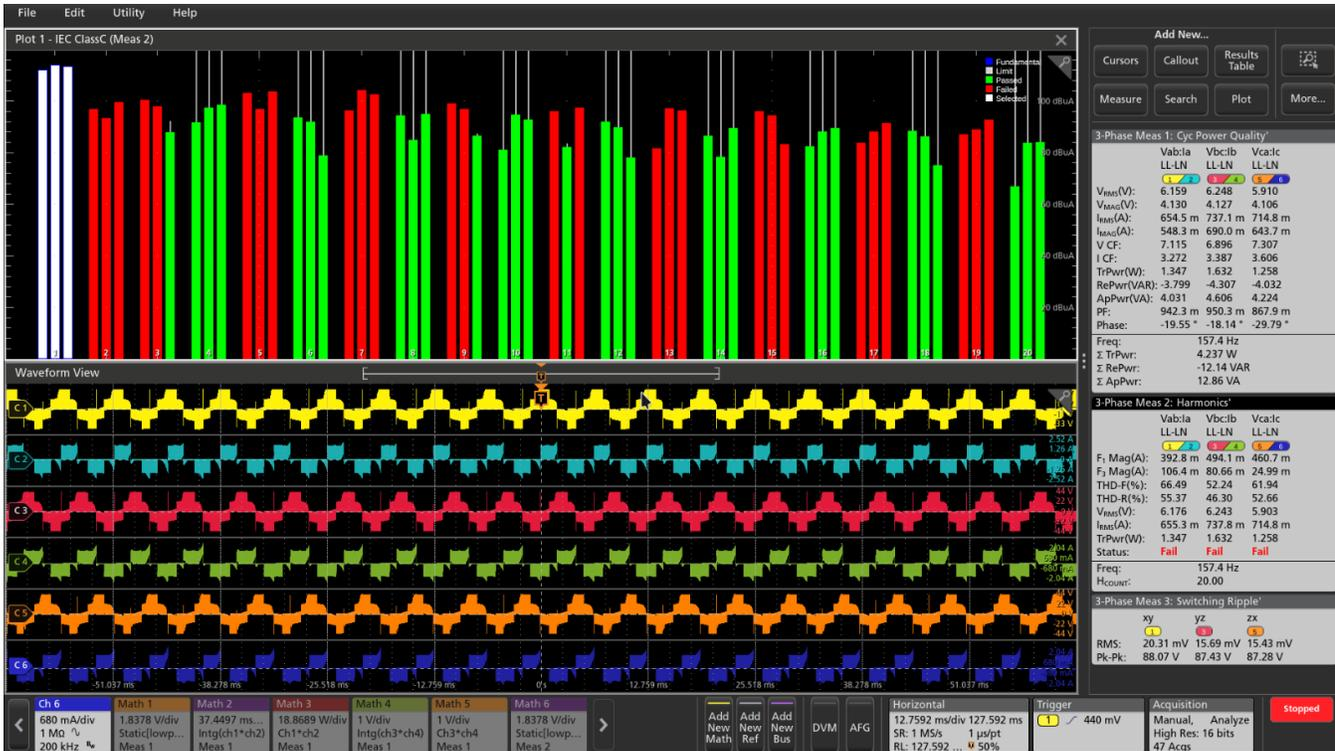
Figure 29: The harmonics plot indicates passing harmonics test results. Each set of bars contains results for phases A, B, and C for easy correlation. The set of green bars indicate a pass and the red bars indicate a fail.
