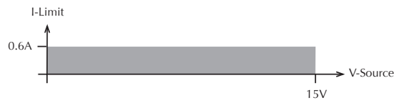
C) 500mA Measurement Range (Model 2303-PJ)
