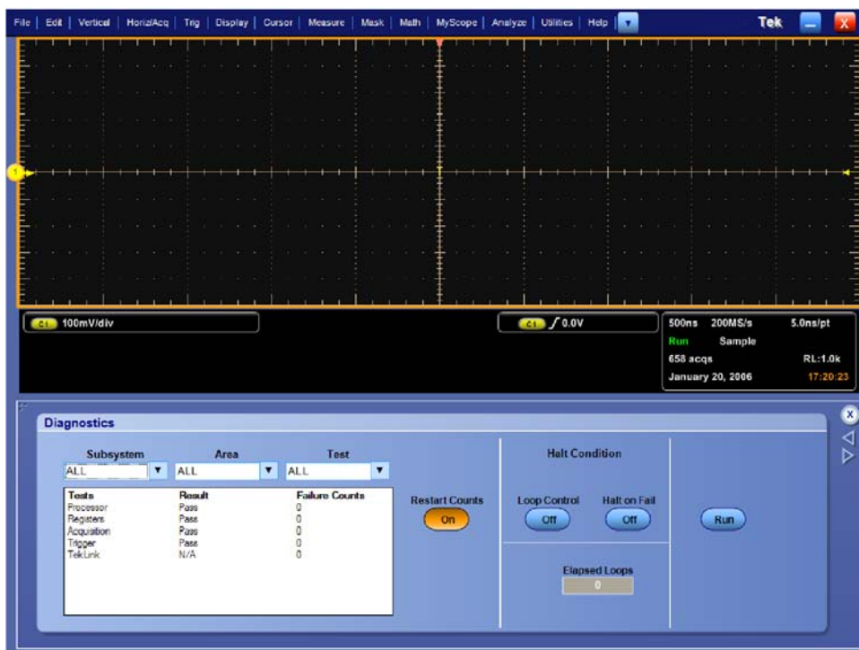
Figure 4-8: Diagnostics control panel
