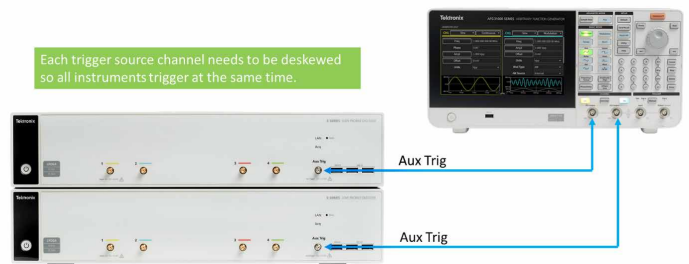
Synchronize multiple instrument channels within 200 ps using manual deskew and the Aux Trigger input
