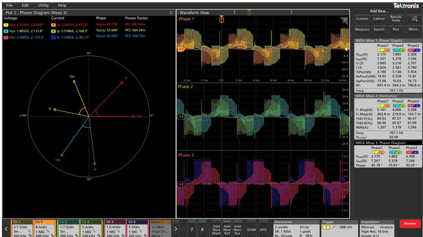
On the left is a Phasor Diagram displaying the phase and magnitude of current and voltage measurements for all three phases of power. In the results badge on the right, are the results from the automated measurements of power quality, power harmonics and the phasor diagram.
