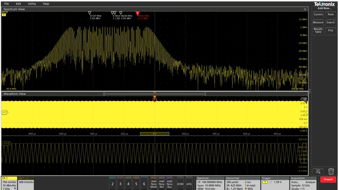
The lower trace is the frequency vs. time trace derived from the input signal. Notice that the Spectrum Time is positioned during a transition from the lowest frequency to the middle frequency, so the energy is spread across a number of frequencies. With the frequency vs. time trace, you can easily see the different frequency hops, simplifying characterization of how the device switches between frequencies.
