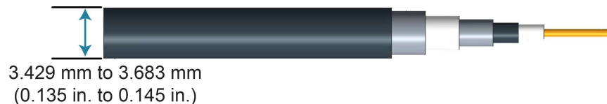
Figure 5: SC-22 triaxial cable dimensions
