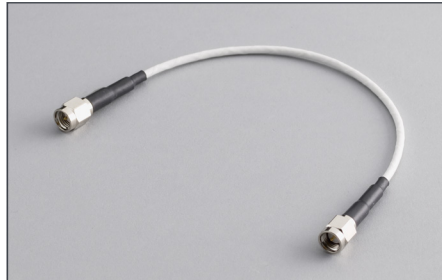
CA-452A: 20.4 cm (8 in) RG188 coax cable terminated with an SMA male plug on each end, 50 \Omega impedance.
