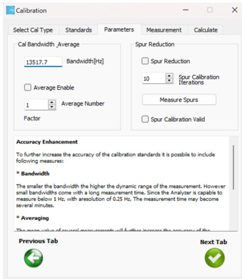
Figure 2-6 Calibration window, Parameters tab
