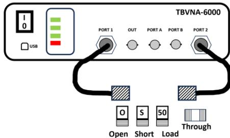
Figure 2-24 setup for full 2-port calibration
