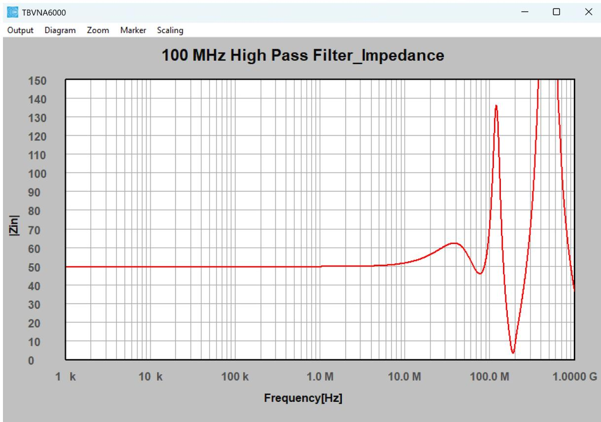
Figure 2-45, measurement result
