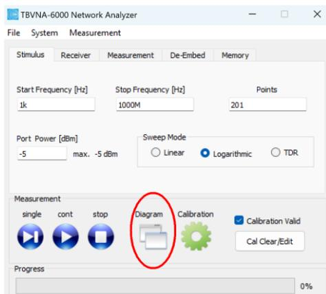
Figure 2-9 Main window, Diagram button
