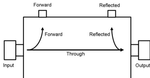
The ports Input/Output and Forward/Reflected can be exchanged. However, directivity may deviate from the documented values.
