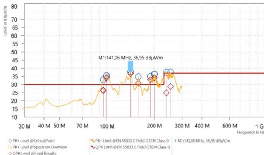
Again QP limits and a peak detector measurement. Now, several spurious cross the QP limits and as QP detector amplitudes are always lower than peak detector amplitudes, there is a chance that the spurious are still below the QP limit line. Consequently, at the frequencies with the highest spurious levels, QP
