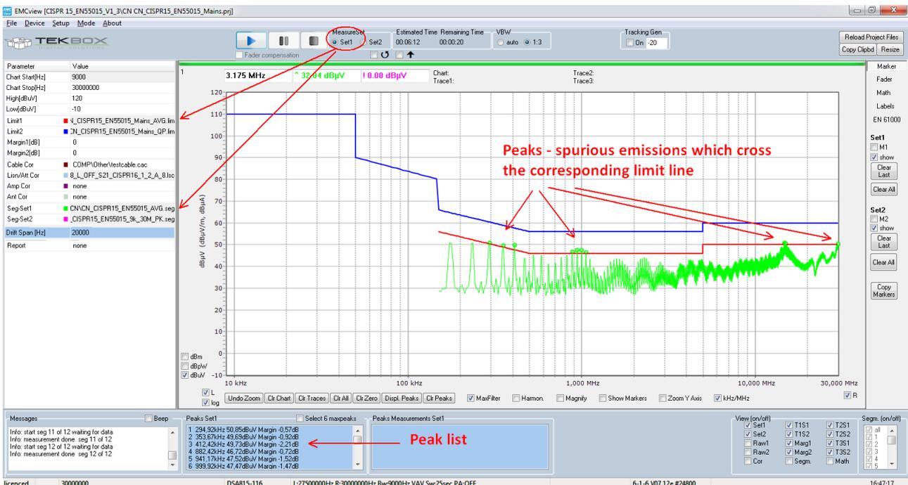
The peaks are displayed in the graph, using marker circles; furthermore the frequencies, amplitudes and offset to the limit line are displayed in the peak list.
