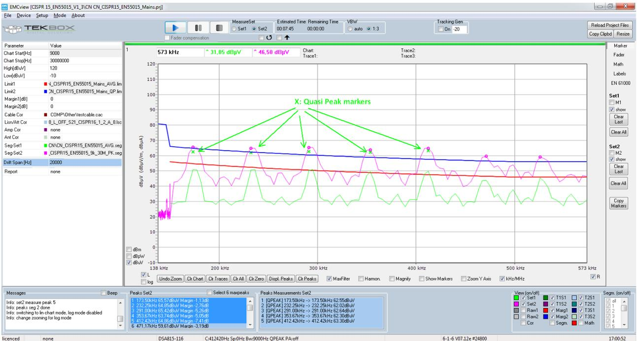
The next screenshots show the frequency range around 15 MHz. The highest point is selected by manually placing a marker. First, pressing the **Clr Marker** button deletes the automatically generated markers. Next a manual marker is placed at the graph and then transferred into the peak list:
