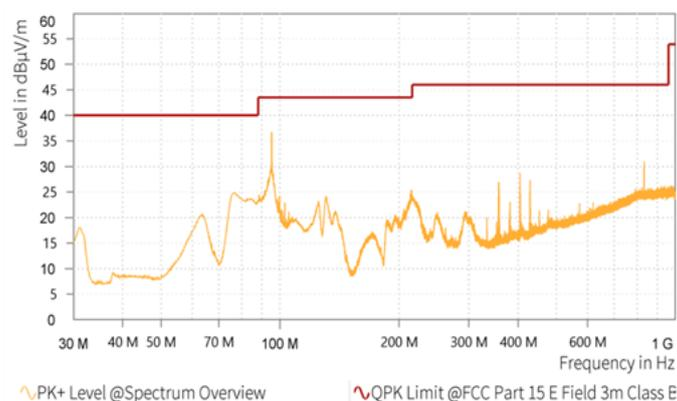
In the legend of the screenshot you can see QP limits, but the measurement was carried out using the peak detector. Peak detector measurement results are far faster than QP measurements and Peak detector measurements always deliver a higher value than QP measurements. As in the above case, the Peak result is not crossing the QP limits, you know that the radiated noise test is passed and there is no need to make a QP measurement.
