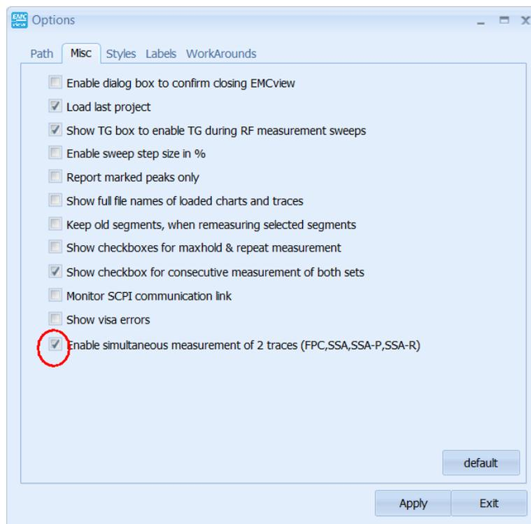
Now, in case that you start the measurement with **Set1** activated, it will simultaneously measure a second graph, using the detector configured in the segment file for **Set2**. Other than that, it will use all settings configured in the segment file for **Set1**. Likewise, if you start the measurement with **Set2** activated, it will
