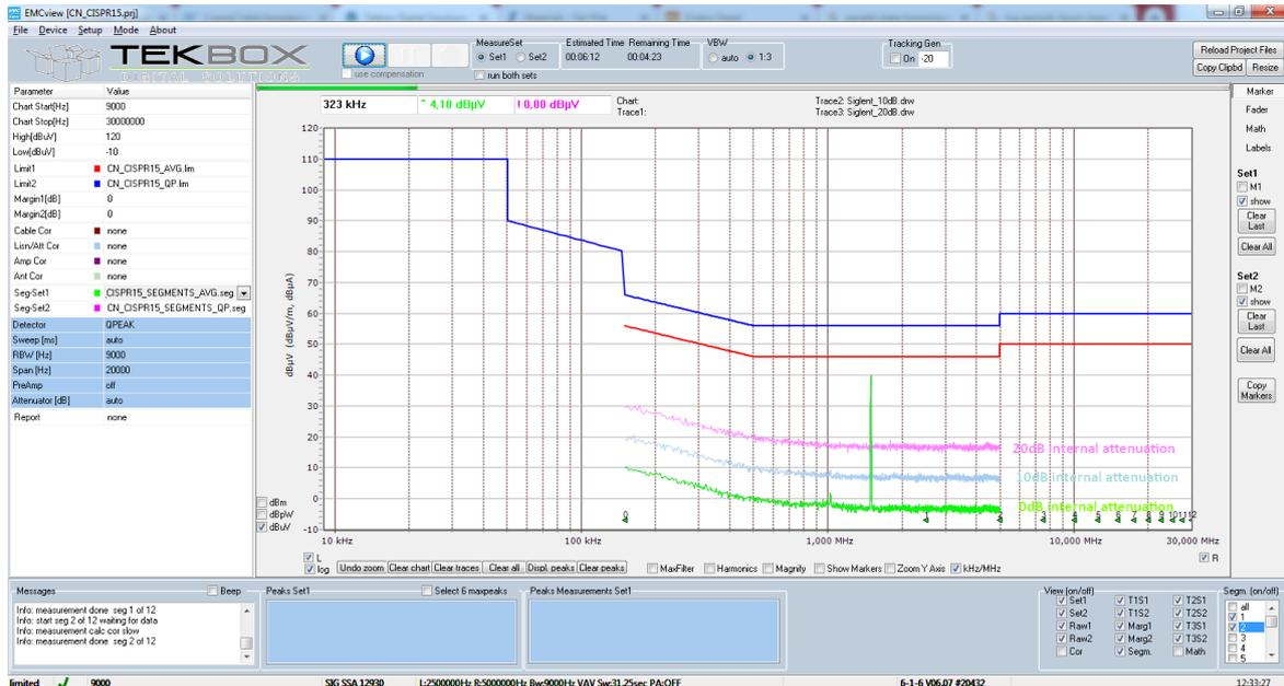
And here the zoomed view. The amplitude values obtained from the analyzer are already compensated with respect to the internal attenuation.
