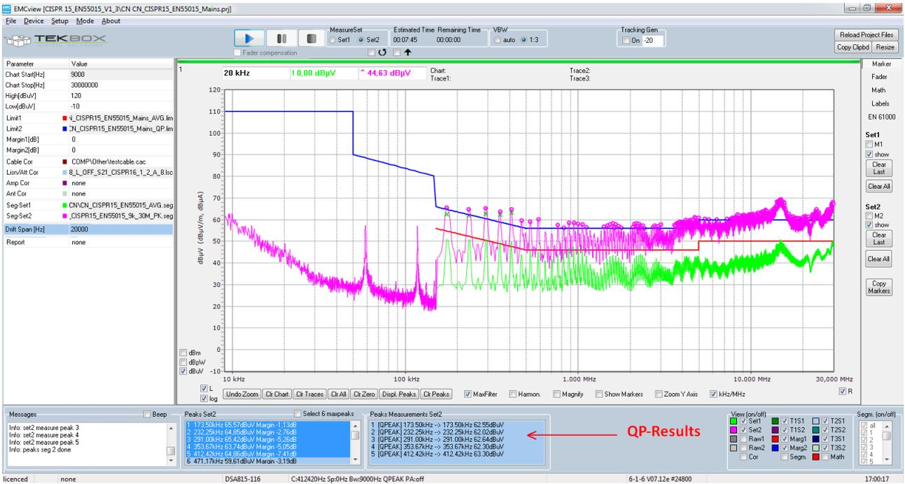
The QP Levels are furthermore displayed in the graph, as can be seen in the zoomed graph of the screenshot below. As expected, the QP results are always in between the levels of the peak and average measurement. The QP re-measurement shows that the first two spurious would pass QP limits with some tiny margin.
