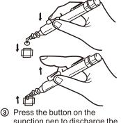
sunction pen to discharge the air, then release the button to produce vacuum suction force to pick up IC.
