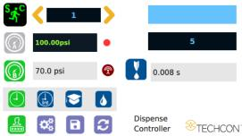
Note: If the sequence mode is set to activate memory cells 1-3 and the delay time is set at 5000 ms, the controller will activate memory 1 to 3 continuously with 5000 ms delay between each activation. The delay time must be at least 15 ms.
