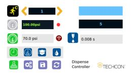
Note: If the controller is set to activate memory cell 1 and the delay time is set at 5000 ms, the controller will activate memory 1 continuously with 5000 ms delay between each activation.
