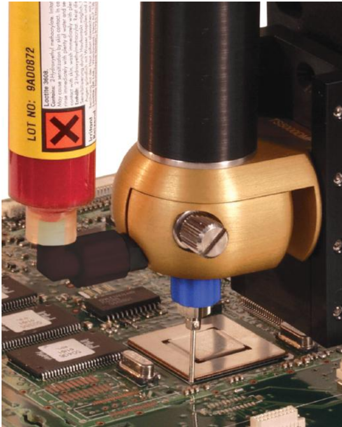
TS5000DMP - Performing underfill
