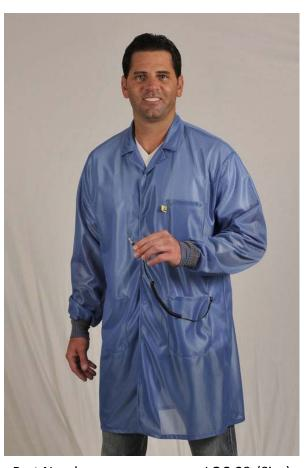
This ESD coat is an effective static shield. The light-weight fabric makes this style one of our most popular garments. Surface resistivity of the fabric is 1X10<sup>5</sup> and the sleeve-to-sleeve resistance of the garment is guaranteed to stay below 3.5X10<sup>7</sup> for 100 washes or 2 years.
