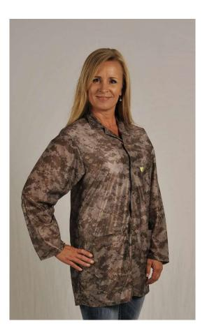
This ESD jacket is an effective static shield. The light-weight OFX-100 fabric makes this style one of our most popular garments. Surface resistivity of the fabric is 1X10<sup>5</sup> and the sleeve-to-sleeve resistance of the garment is guaranteed to stay below 3.5X10<sup>7</sup> for 100 washes or 2 years.
