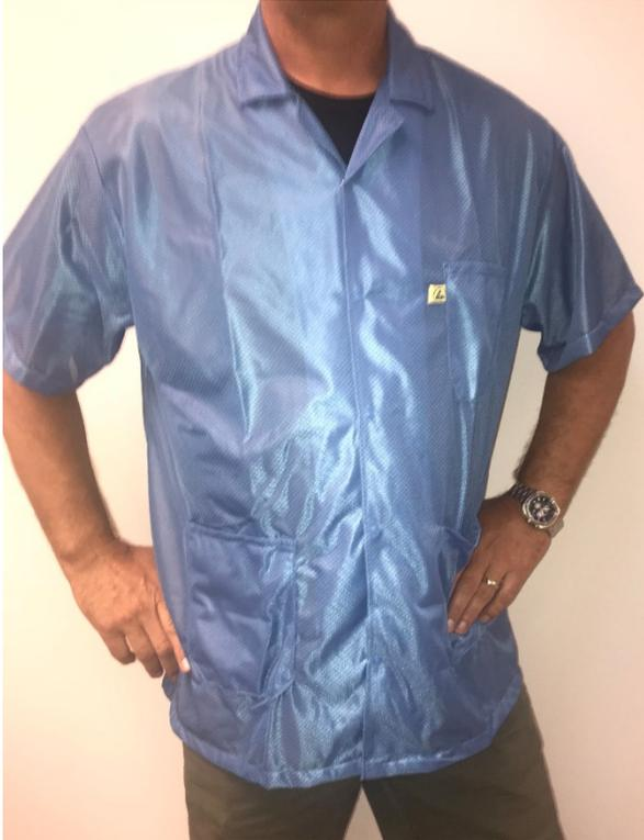
This ESD jacket is an effective Category 1 static shielding ESD garment. The light-weight OFX-100 fabric makes this style one of our most popular garments. Surface resistivity of the fabric is  $1 \times 10^5$  and the sleeve-to-sleeve resistance of the garment is guaranteed to stay below  $3.5 \times 10^7$  for 100 washes or 2 years.
