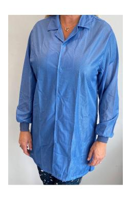
This ESD jacket is designed to ground the wearer through the garment through the ESD knit cuff and a ground cord connected at the side seam snap. This allows for handsfree movement without tethering one hand, which is required when using a wrist strap connected to a ground cord.
