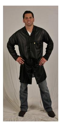
This ESD coat is a Category 2 groundable garment. The light-weight fabric makes this style one of our most popular garments. Surface resistivity of the fabric is 1X10<sup>5</sup> and the sleeve-to-sleeve resistance of the garment is guaranteed to stay below 3.5X10<sup>7</sup> for 100 washes or 2 years.
