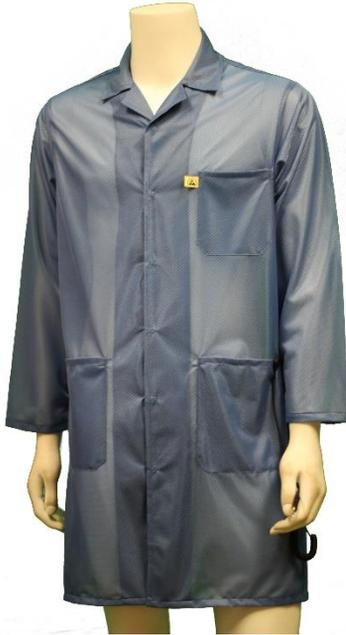
This ESD coat is designed to ground the garment and the wearer through a ground cord connected at the hip pocket snap. This allows for hands-free movement without tethering one hand, which is required when using a wrist strap connected to a ground cord.
