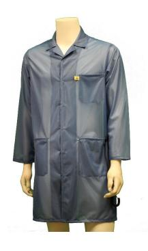
This ESD coat is designed to ground the garment and the wearer through a ground cord connected at the hip pocket snap. This allows for handsfree movement without tethering one hand, which is required when using a wrist strap connected to a ground cord.
