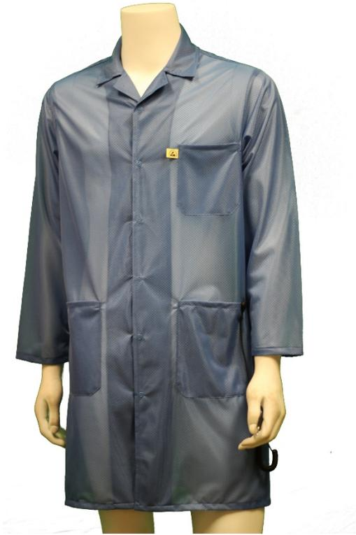
This ESD coat is a Category 2 groundable garment. The light-weight fabric makes this style one of our most popular garments. Surface resistivity of the fabric is  $1 \times 10^5$  and the sleeve-to-sleeve resistance of the garment is guaranteed to stay below  $3.5 \times 10^7$  for 100 washes or 2 years.
