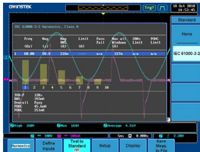
Figure 5: The GDS-3000 Harmonics function
