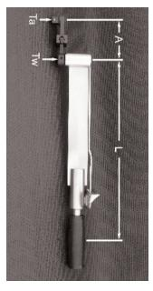
The applied torque with an adapter or extension that changes the effective length of the tool is the sum of the length of the change plus the lever length of the wrench. This is shown in the formula below.
