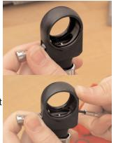
Step 18 Insert snap ring. Assembly is complete when snap ring has been inserted.
