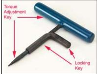
CART Tool for presetting torque.
