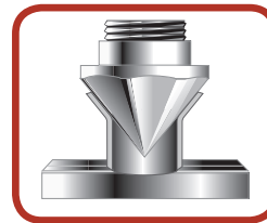
Flares rolled out above die bar by super-smooth faceted cone. Makes stronger, highly polished flares.
