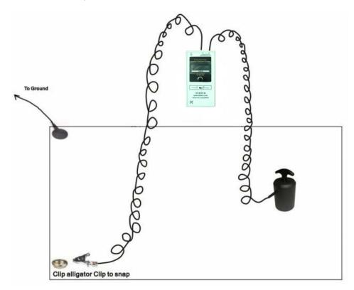
Attach the alligator clip to the lead and connect it to the ground snap or connect the banana plug to a common point ground plug:
