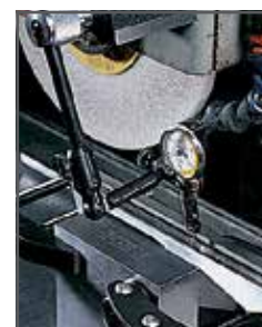
657A with 711LS Last Word Dial Test Indicator setting up workpiece on surface grinder.
