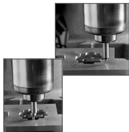
Above: Locating the center with 827MB Left: Locating the edge of a part with 827MA
