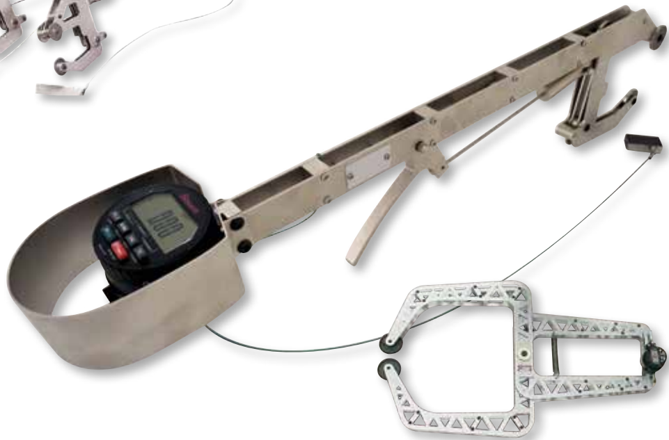
Variation on a theme: A large caliper with long reach for web thickness of train tracks hot or cold.
