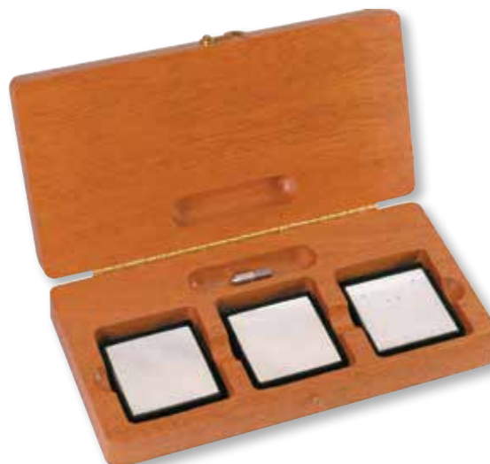
PT05272 HRC 3-Block Master Calibration Kit
