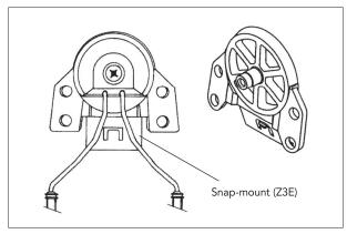
positions: working position, ventilation position and parking position. When in use, the cups must be placed in working position. Press the wires inward until you hear a click on both sides. Make sure that the cup and the headband wire in working position are not pressing on the helmet lining or the edge of your hardhat so that leakage can occur. Parking position should not be used if the cups are damp inside after an intense period of use.
