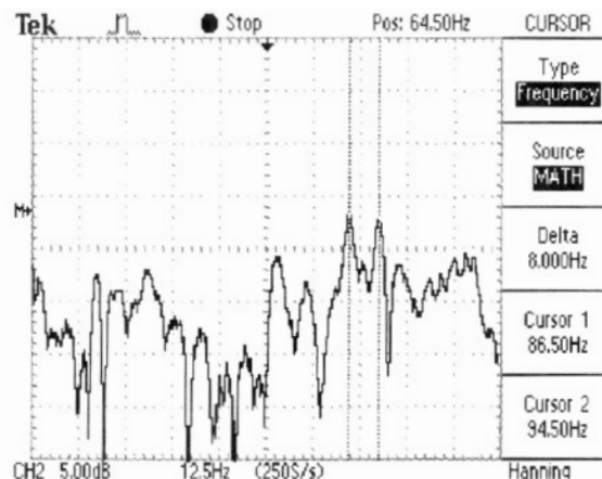
Figure 8. FFT plot of the vibrations occurring on the roof beam during simulated vehicle movement.
