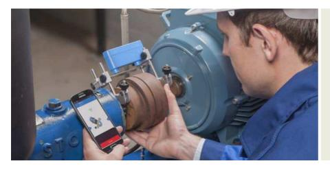
Shaft alignment is recommended for almost every industry, as it enables machine uptime to be significantly improved and maintenance costs to be reduced.
