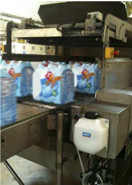
For lubrication of chains in packaging machines, palletizers, shrink wrapper, etc.
