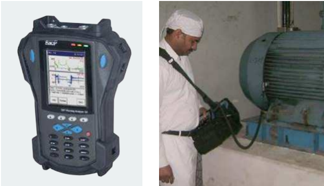
Periodic data collection with SKF Microlog Analyzer
